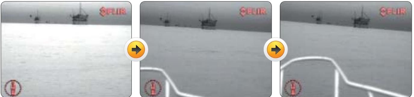
Gyro stabilised imager; target still in view despite bow rise and fall
